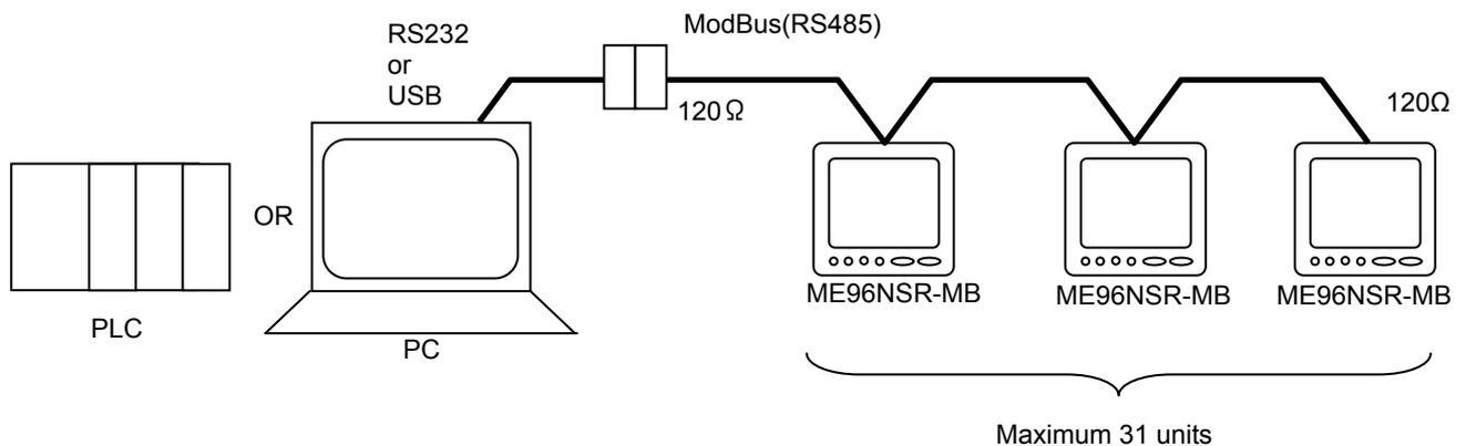
※ME96NSR-MB performs a termination of 120 ohm resistance by short-circuiting the terminal of T/R- and Ter.
