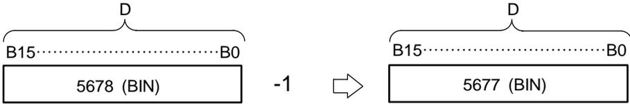
(2) If DEC is executed when the details of the device designated with D are 0, -1 will be stored in the device designated with D.
