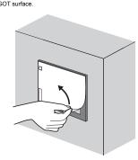
2) Peel the release paper off the back of the new protective sheet. Position the hole for the USB environmental protection cover of the sheet to the USB environmental protection cover of the GOT. If the protective sheet without the hole for the USB environmental prover is attached, position the sheet from the upper left of the GOT.
