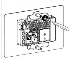
**NOTE:** If you exceed the recommended torque when tightening the installation fastener's screws, the front of this product may become distorted.
