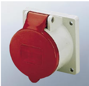
▲ IP 44 panel-mounted receptacle, straight, screwless spring terminal technology TwinCONTACT connecting terminals suitable for through wiring.
