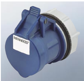
▲ IP 44 RAPIDO panel-mounted receptacle for wall opening 61 mm diameter, central fastening, screwless spring terminal technology TwinCONTACT connecting terminals suitable for through wiring.
