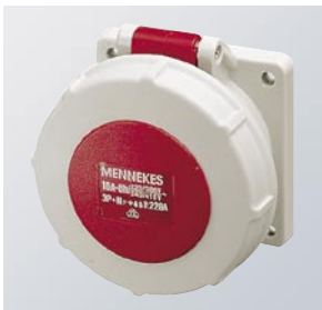
▲ IP 67 panel-mounted receptacle, straight, screwless spring terminal technology TwinCONTACT connecting terminals suitable for through wiring.
