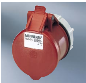
▲ IP 44 RAPIDO panel-mounted receptacle for wall opening 70 mm diameter, central fastening, screwless spring terminal technology TwinCONTACT connecting terminals suitable for through wiring.
