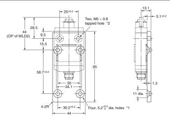
Note: Four hexagonal flat head bolts  $(M5 \times 0.8, length: 10)$  and two Allen-head bolts  $(M5 \times 0.8, length: 10)$ length: 15) are included.
