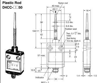
\*1. Operation is possible in any direction except parallel to the axis **4.**\*2. The ideal range for operation is between the tip of the rod and 1/3 of the length of the actuator.
