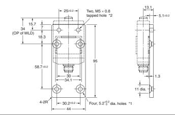
Note: Four hexagonal flat head bolts (M5  $\times$  0.8, length: 10) and two Allen-head bolts (M5  $\times$  0.8, length: 15) are included.
